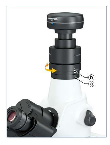
9. Adjusting the Parfocality **between Observation** Image and Camera Image
