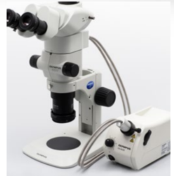
Coaxial reflected light illuminator / SZX2-ILLC10
