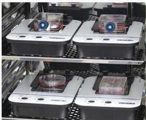
Compact design fits in standard-sized incubators; no special preparation is needed for installation
